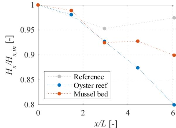
Figure 2 - Normalized wave heights  $H_s/H_{s,in}$  over the length of the surrogate models  $x$  normalized by the wave length  $L$ .
