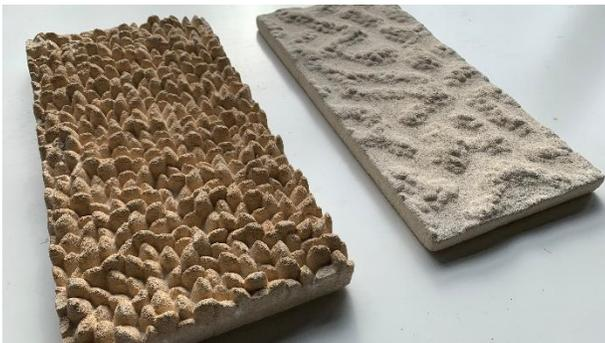
Figure 1 - Surrogate model tiles (0.50 x 0.25 m) of a Pacific oyster reef (left) and a blue mussel bed (right).
