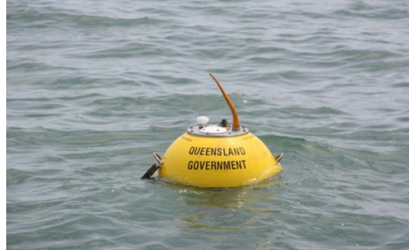
Figure 2 DWR wave monitoring buoy deployed off Palm Beach, Queensland.
