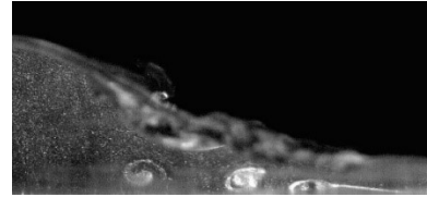
Figure 4 - Example of bed-generated eddies during the downwash revealed by the seeding particles in the HSPIV raw image
