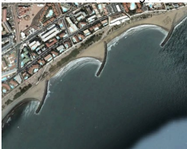
Figure 1- Beach stabilization with hard structures
