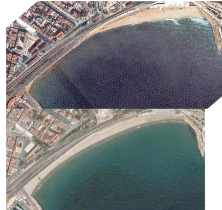
Figure 3 - Beach shoreline variation due to changes in wave conditions
