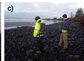
Figure 1: Photo of the mounted Lidar monitoring a single cross-shore line of the revetment at low tide, a) and high tide b). c) Photo of particle tracking survey using RFID detection and GPS.
