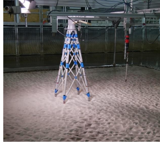
Figure 1. Photo of the experimental setup and the used Jacket structure.
