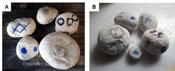
Figure 4 - Pebbles of set B: a) after 2000 revolutions; b) Pebbles after 5000 revolutions
