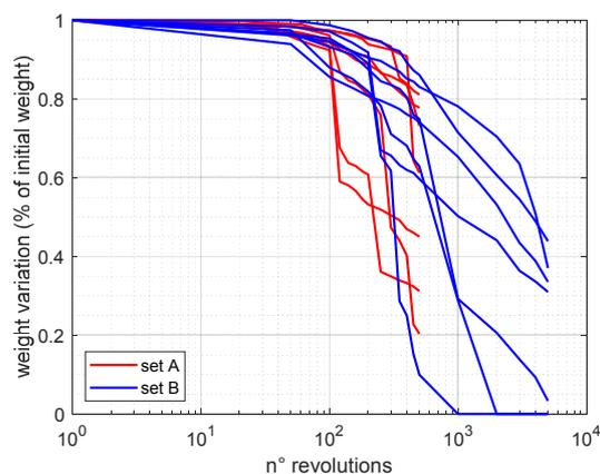
Figure 5 - Weight variation (ratio between the final weight and the initial weight) of the pebbles for the two tested sets
