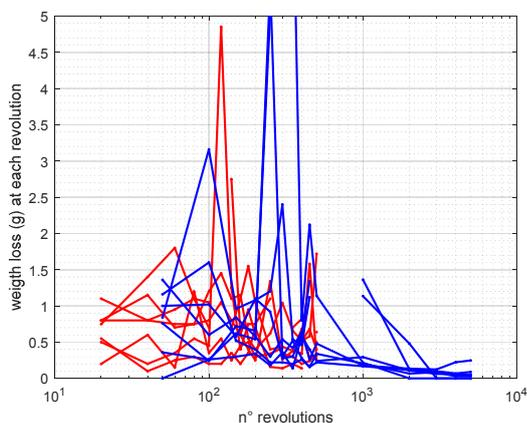
Figure 6 - Pebbles weight loss after each revolution (g/revolution) for the two tested sets
