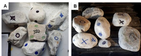
Figure 3 - Pebbles of set B: a) before the tumbling experiment; b) after 500 revolutions
