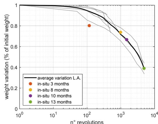
Figure 7 - Comparison between weight variations of the non-broken pebbles tested in the L.A. machine with the one measured by Bertoni et al. (2016)
