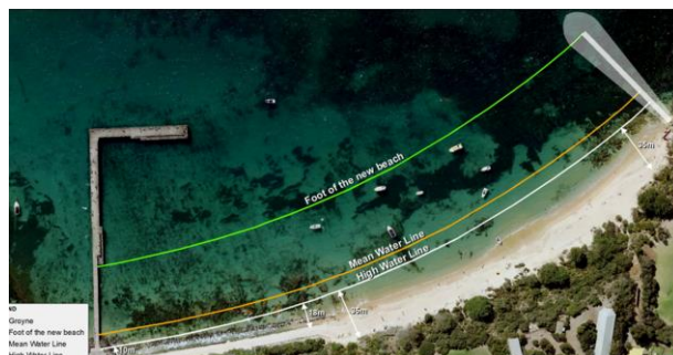
Figure 11 - Schematisation of the proposed groyne and renourished beach.
