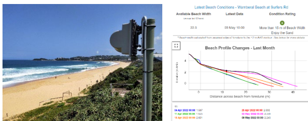
Figure 4 - Application of real-time, continuous Lidar beach monitoring system and web interface.
