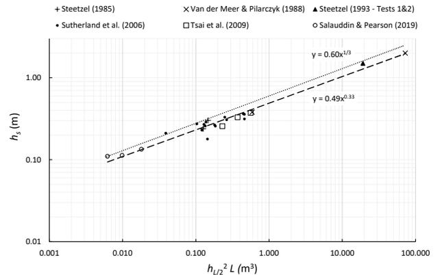
Figure 2 - Moveable bed model scour depth data plotted as a function breaking wave energy.
