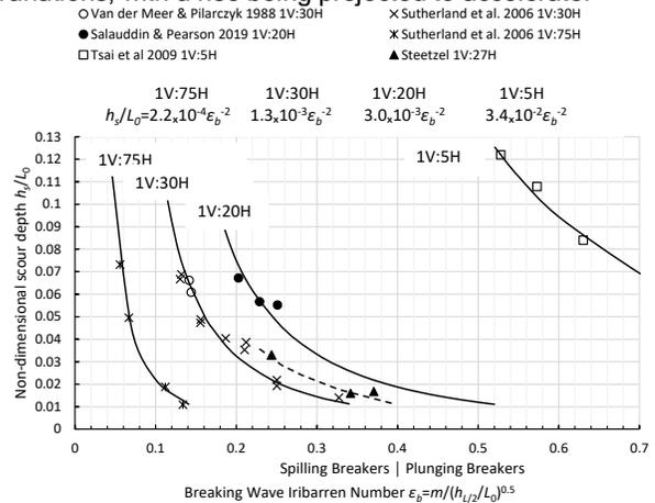
Figure 3 - Relationships between scour depth and Iribarren Number for various beach slopes from this study data.
