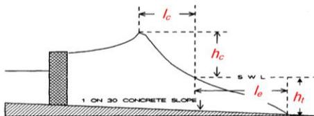
Figure 1 - Characteristic dimensions of a dynamic revetment (modified from Ahrens, 1990).
