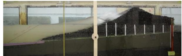
Figure 2 - Reshaped dynamic revetment structure due to incoming wave action causing gravel transport to the crest.
