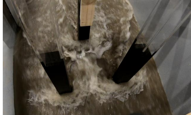
Figure 1 - Bore impact on three-structures setup
