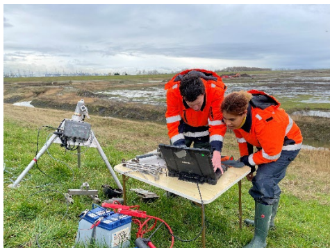
Figure 1 - Set-up of grass sod pulling tests
