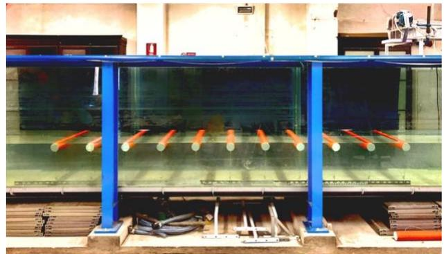
Figure 2 - Experimental setup: 11 cylindrical pendula with a mutual distance  $L = 0.35$  m
