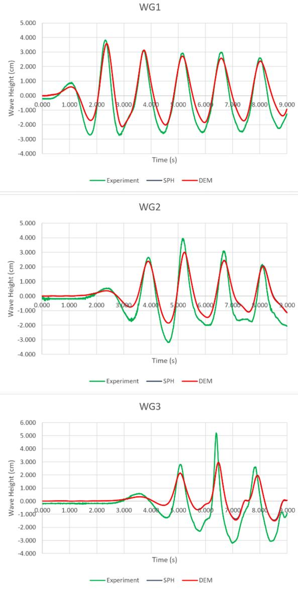
Figure 4 - Wave Heights at the three points in the two-dimensional cross-sectional channel
