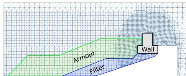
Figure 2: Model mesh and revetment cross-section.
