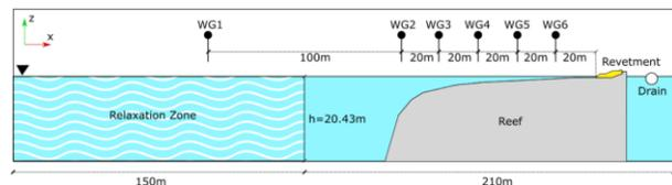
Figure 1: Sketch of numerical wave flume. Note: z axis is out of scale for illustration purposes.
