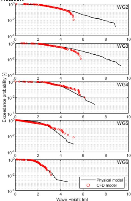
Figure 5: Exceedance probability of wave heights at WG2, WG3 and WG5. The legend applies to all figures. Note: Data from the numerical model are not exact but extracted from a figure.
