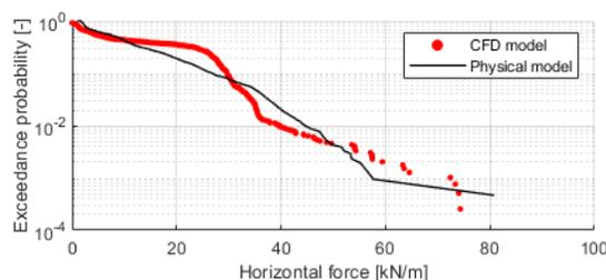
Figure 6: Exceedance probability of horizontal force on the concrete wall. Note: Data from the numerical model are not exact but extracted from a figure.
