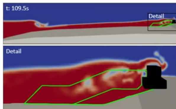
Figure 4: Top: Wave breaking on the reef. Bottom: Example of overtopping.
