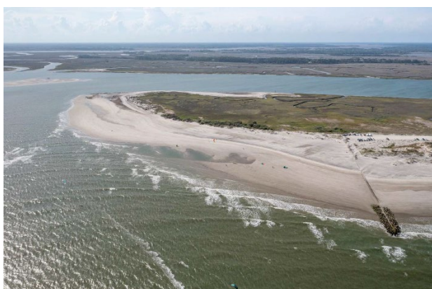
Figure 4 - Downdrift spit at Folly Beach County Park on 3 May 2022, nine years after groin installation. Note the continuous dry sand beach. Photo courtesy of GEL Inc, Charleston, SC.
