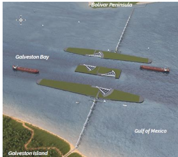
Figure 2: Bolivar Roads Gate System Overview.
