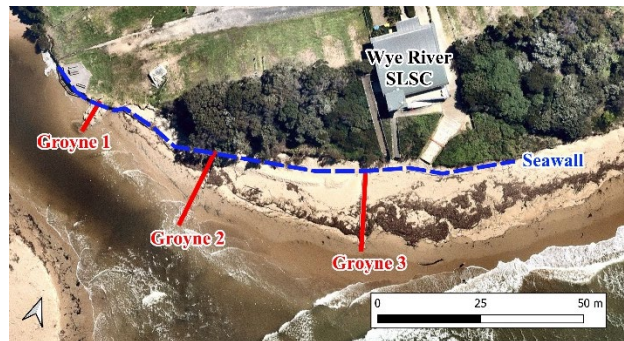
Figure 2 - Installed geo-container structures.
