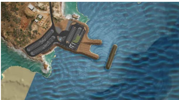
Figure 1 - Example of model output from MIKE21BW phase resolving model at the site (water surface elevation)
