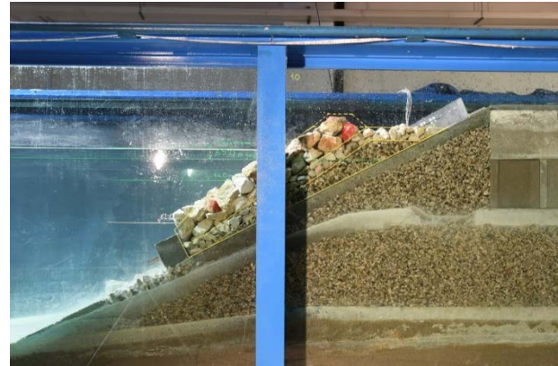
Figure 4b. Configuration B (modified solution). The first large stone above the berm is 2-3 t.
