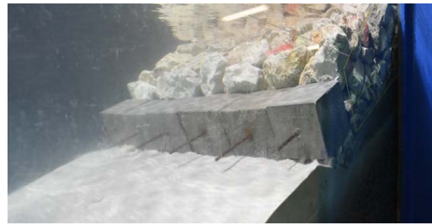
Figure 5 -Barrier in mobile bed wave flume (Config. A).
