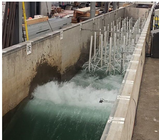
Figure 5 - Testing wave-mangrove-wall interaction for the high-density forest, regular waves and a local water depth of h_i=1.03 m.
