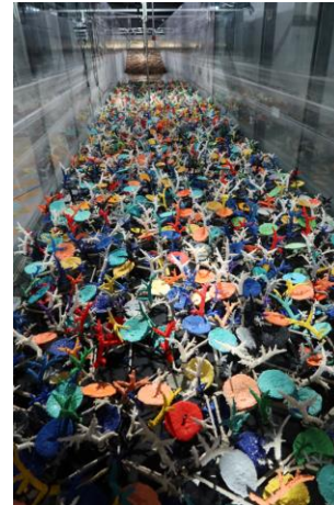
Figure 1 - 8m long and 1.5m wide reef of MARS Inc. reef stars with 3D Printed corals attached within the University of Western Australia Coastal and Offshore Engineering Laboratory wave flume
