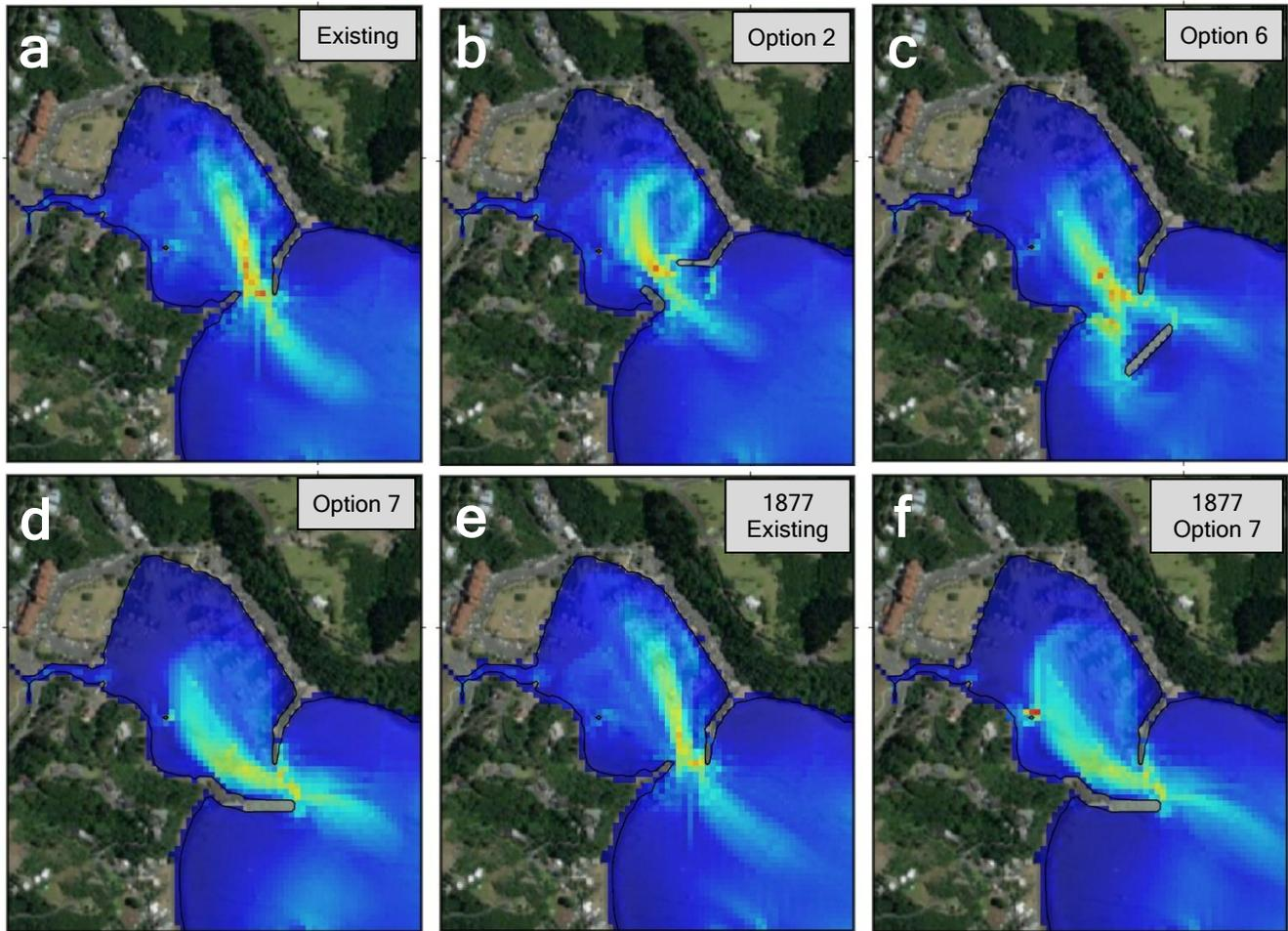
Figure 4 Comparison of model output. Panels a-d compare the 1976 scenario over 4 different configurations. Panels e and f compare the present-day configuration to Option 7 for the 1877 tsunami from northern Chile.
