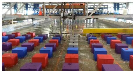
Figure 1 - Photo of the experimental setting with partial wall in front of the structural array.
