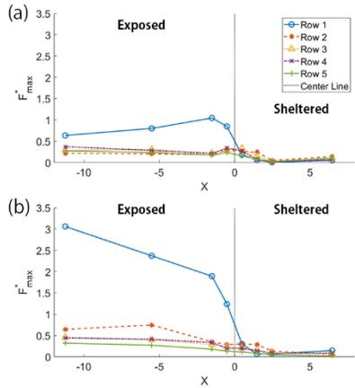
Figure 2 - Maximum dimensionless quasi-static loads for (a) error function waves with inundation and (b) solitary waves with inundation.
