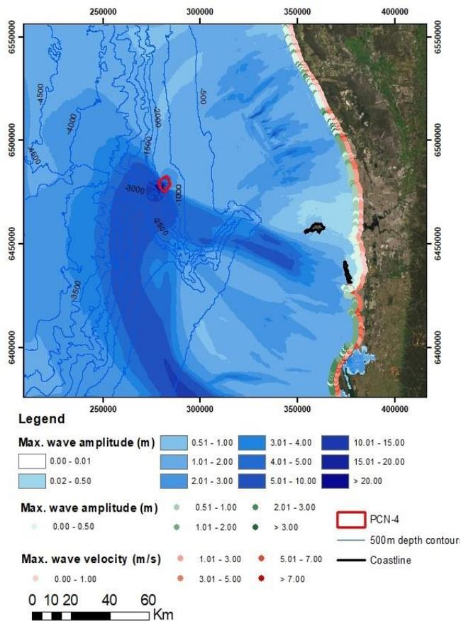
Figure 1 - PCN4 maximum wave amplitude and inundation 2.5 hours after initial failure.
