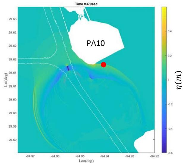
Figure 5 - Screen shot of FUNWAVE simulation results for free-surface elevation  $\eta$  generated by the same inbound deep-draft oil tanker shown in Figure 4 (L: 244m, B: 42m, D: 10m, U=10m/s). The location of the field measuring station is indicated by the red dot.
