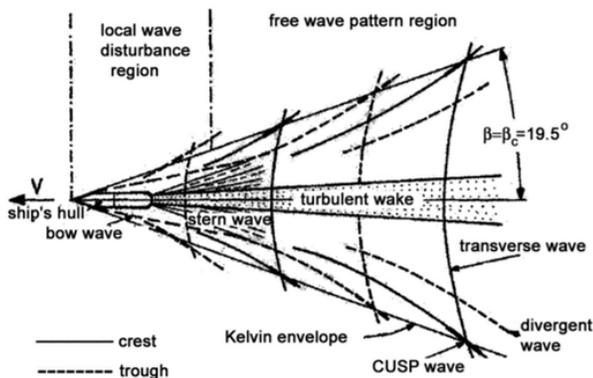
Figure 1 - Geometry of Kelvin ship wake components including bow, stern, transverse, and divergent waves (Hennings et al., 1999).
