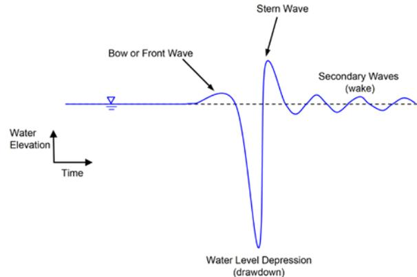
Figure 2 - Typical time series of water free surface fluctuation produced by a large moving vessel (Hennings et al., 1999).
