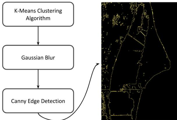
Figure 2 - Flow chart outlining the shoreline detection algorithm. We first separate the image into land and water using the K-Means algorithm. Then we apply a blur to the image before detecting the edge between the land and water clusters. The image to the right is the output.
