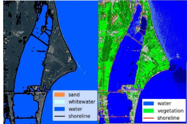
Figure 3 - Aerial image of Cape Canaveral, FL in two parts: Left is what CoastSat produced by default, where sand is represented in orange, whitewater in light blue, water in blue, and shoreline is the black line. Right includes our NDVI component of the CoastSat process, and shows the refined coastline algorithm (red line), the water (blue), and the vegetation density (green, with brighter green more vegetation).
