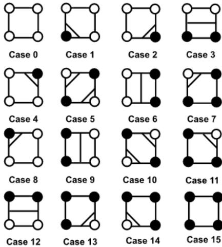
Figure 1 - The 16 topological cases of cells in the Marching Squares Algorithm. Filled circles represent 1's while hollow circles represent 0's, and 4 pixels are considered at a time. The algorithm goes through all the pixels in an image and at the end, the lines created from the 16 topological cases create the extracted shoreline [12].
