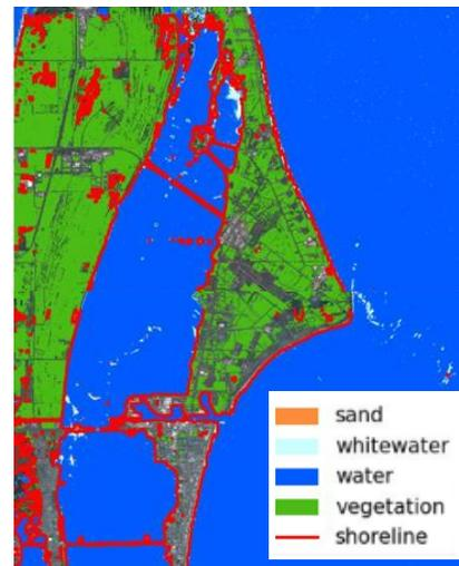
Figure 4 - Final output of CoastSat with the added Canny Edge Detection and vegetation index. The image shows a satellite view of the shoreline of Cape Canaveral, FL. Sand is represented in orange, whitewater in light blue, water in blue, vegetation in green, and shoreline is the red line.
