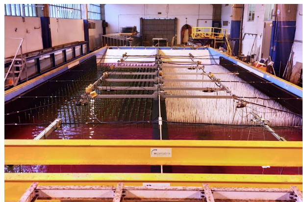
Figure 1 - Experimental set-up. Mangrove mimics at the left side and saltmarsh mimics at the right side. The smooth rigid slope covered with white vinyl is at the end of the wave tank and pink water can be observed due to the use of rhodamine for dyeing.
