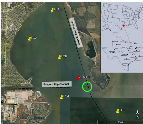
Figure 1 - Confluence of the two channels (Bayport Flare, highlighted in green) within the Upper Galveston Bay, Gulf Coast, TX. Colored pins show the locations of fixed ADCP deployments (red) and TCM (yellow)
