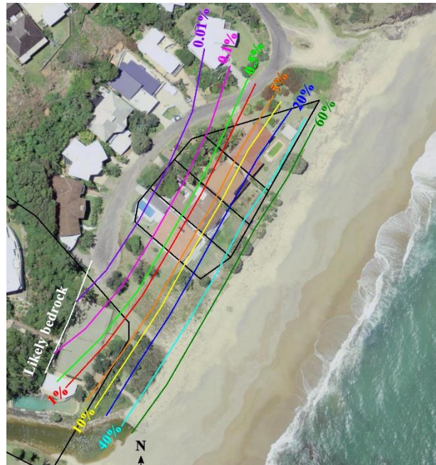
Figure 1 - Example of probabilistic coastal hazard lines in an erosion/recession context, for a particular year (for CBA, these discrete probabilities would most conveniently be provided to the economist as a continuous relationship between landward distance and probability)
