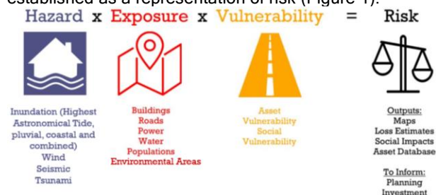
Figure 1 - risk, represented by direct financial losses, were calculated through a function of hazard intensity at the location of each asset in the exposure database and the vulnerability of the asset to damage relative to each hazard.
