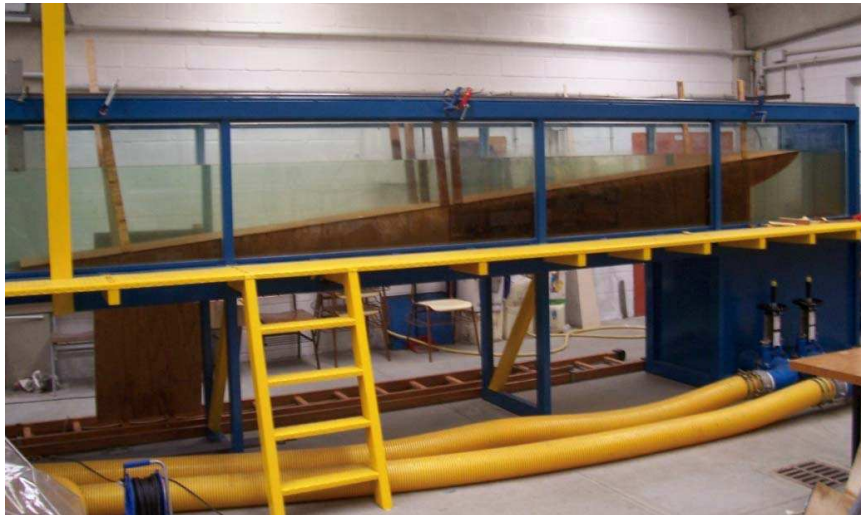
Figure 8. Wave dissipation ramp at the downwave end of the flume.
