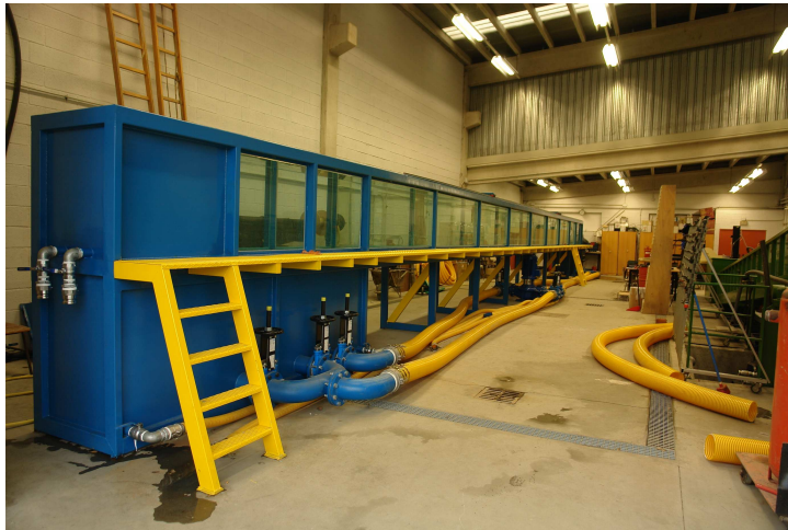
Figure 4. Wave flume at the University of Santiago de Compostela.
