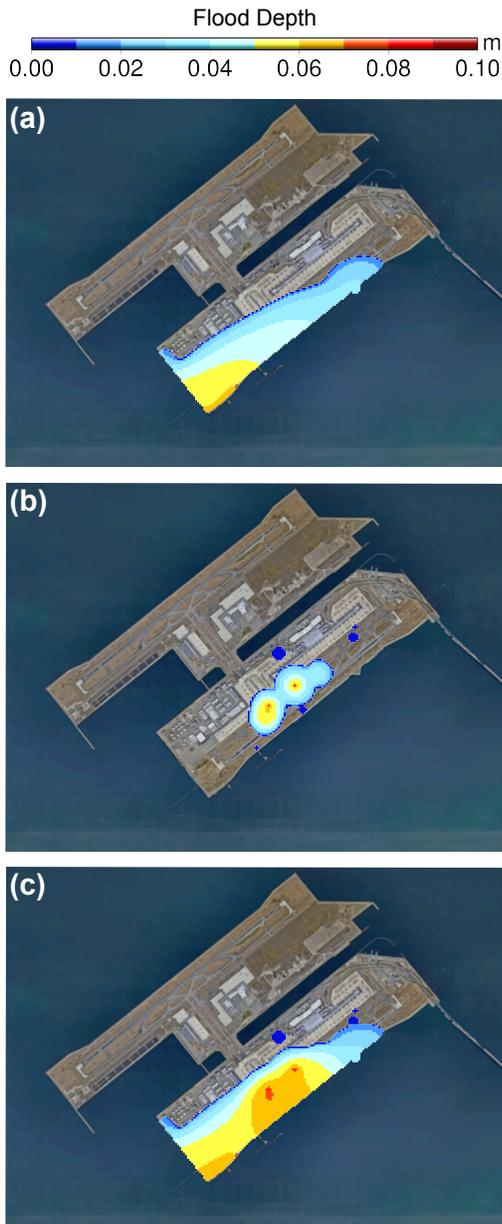
Figure 3 - A flood distribution at 15:10 4th September 2018 (JST) due to each flood component: (a) wave overtopping, (b) reverse flow, and (c) compound components
