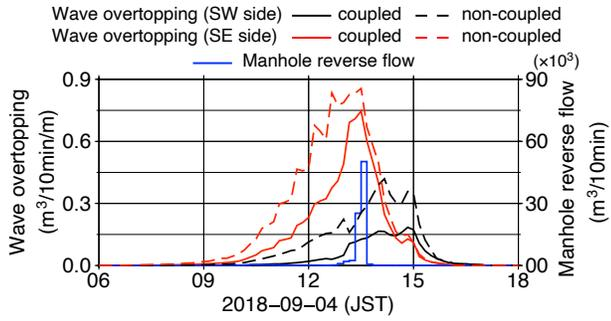
Figure 2 - The amount of flood discharge due to the each component in the coupled and non-coupled simulations
