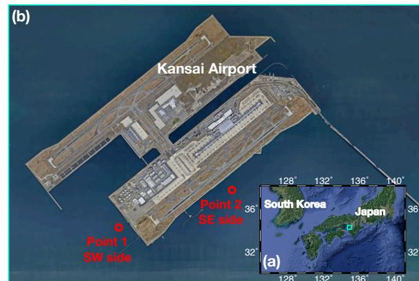
Figure 1 - General layout of Kansai Airport with locations for a comparison of storm surges and waves; Point 1: SW side and Point 2: SE side, 150 m from the breakwaters. (a) a location of Kansai Airport, (b) Kansai Airport
