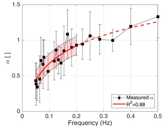
Figure 1: Wave velocities attenuation for each frequency
