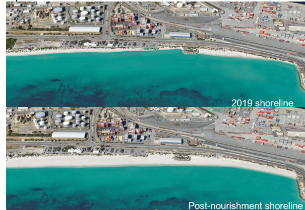
Figure 2 - Oblique Aerial Image of 2019 shoreline (top) and artistic impression of post-nourishment shoreline (bottom)
