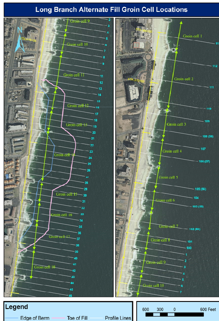
Figure 2. Profile lines and groin cell numbering system.
