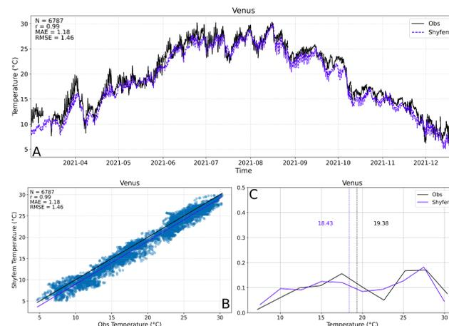
Figure 2 - Temperature measurements (in black) and Shyfem results (in blue) at the Venus station. A) Plot of the 2021 time series of observations and model results. B) Scatter plot of observation and model results. C) PDFs of observations and model results.
