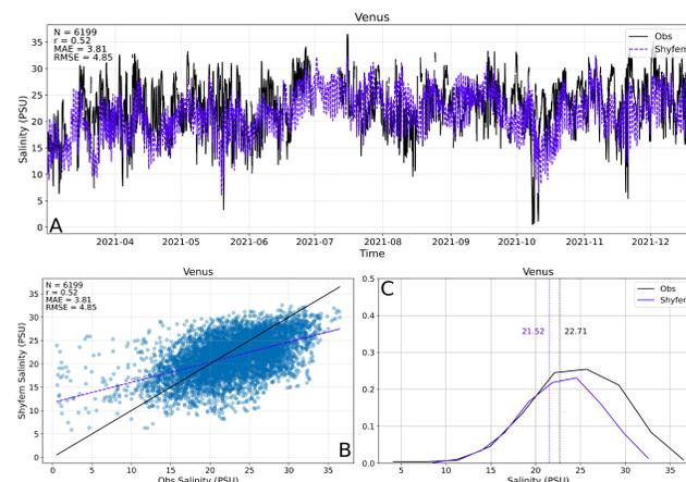
Figure 3 - Salinity measurements (in black) and Shyfem results (in blue) at the Venus station. A) Plot of the 2021 time series of observations and model results. B) Scatter plot of observation and model results. C) PDFs of observations and model results.
