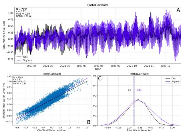
Figure 4 - Sea level measurements (in black) and Shyferm results (in blue) at the Porto Garibaldi station. A) Plot of the 2021 time series of observations and model results. B) Scatter plot of observation and model results. C) PDFs of observations and model results.
