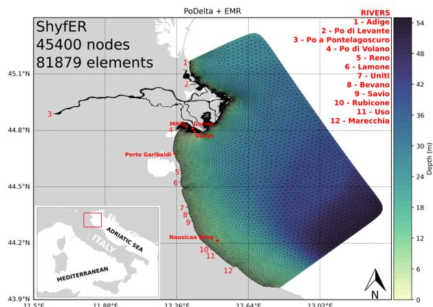
Figure 1 - numerical domain presenting the grid characteristics, most important coastal stations used for calibration and the rivers set as hydrologic boundary conditions.
