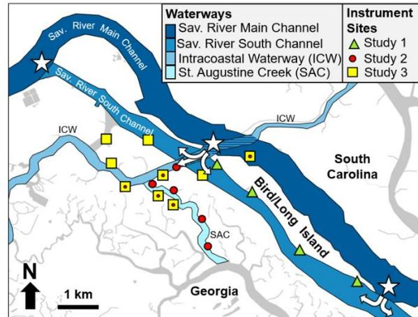
Figure 1 - Instrumentation near the Savannah River, Georgia, USA with potential wake sources (stars) and propagation directions (arrows) into secondary channels.
