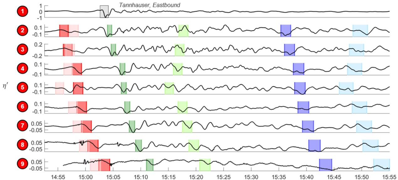
Figure 5 -Time of series  $\eta'/\max(\eta_1)$  showing the arrival time windows of wake propagating from various sources to the instrument array in SAC.
