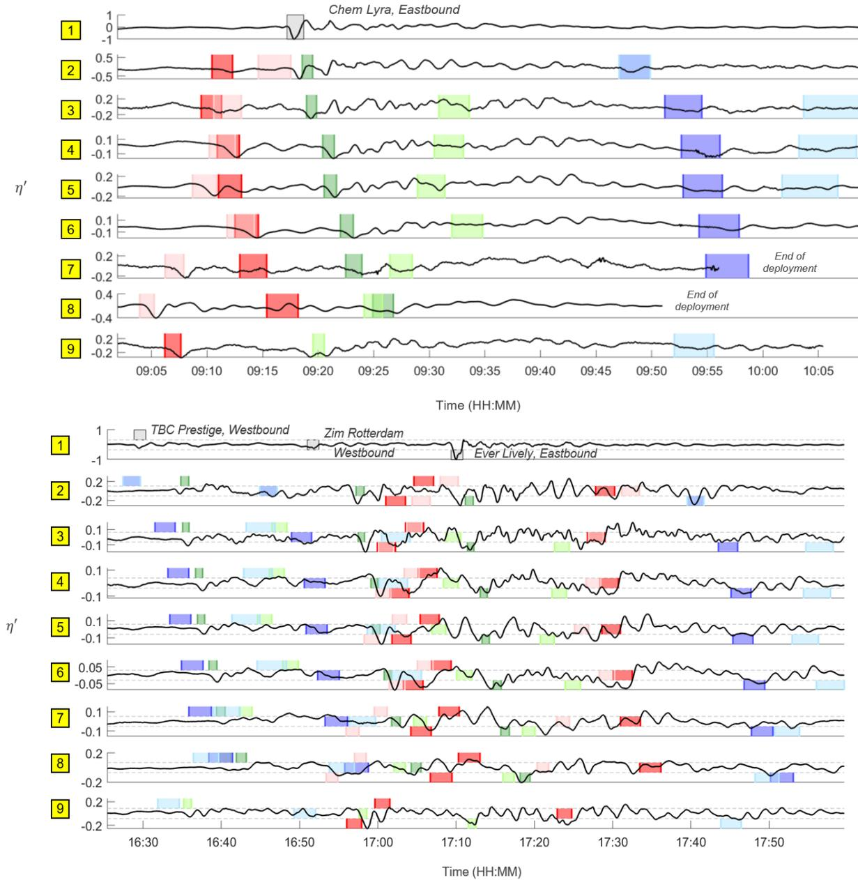
Figure 3 -Time of series  $\eta/\max(\eta_1)$  showing the arrival time windows of wake propagating from various sources for (upper) one isolated vessel passage and (lower) the coinciding passages of three vessels.
