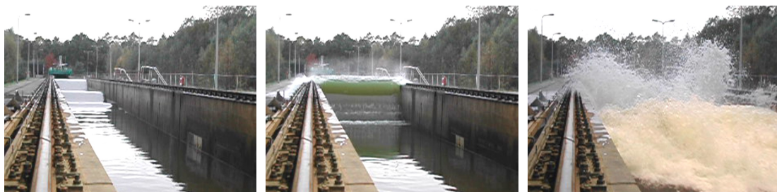
Figure 6. Focussed wave with H_{max} = 3.05 m in de Delta Flume.
