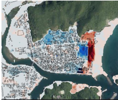
Fig. 5 Maximum inundation height (difference diagram) Fig. 7 Maximum inundation height less than 3.5m (Left: Case A, Right: Case E)
