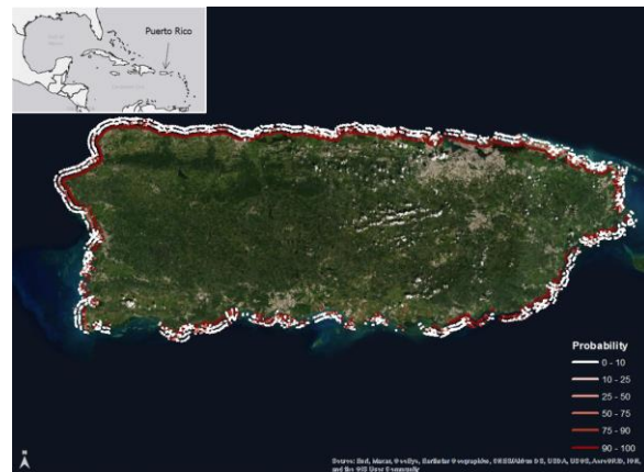
Figure 1 - Probability of hurricane-induced coastal erosion hazards for category 1 storm can be accessed through the USGS Coastal Change Hazards Portal .
