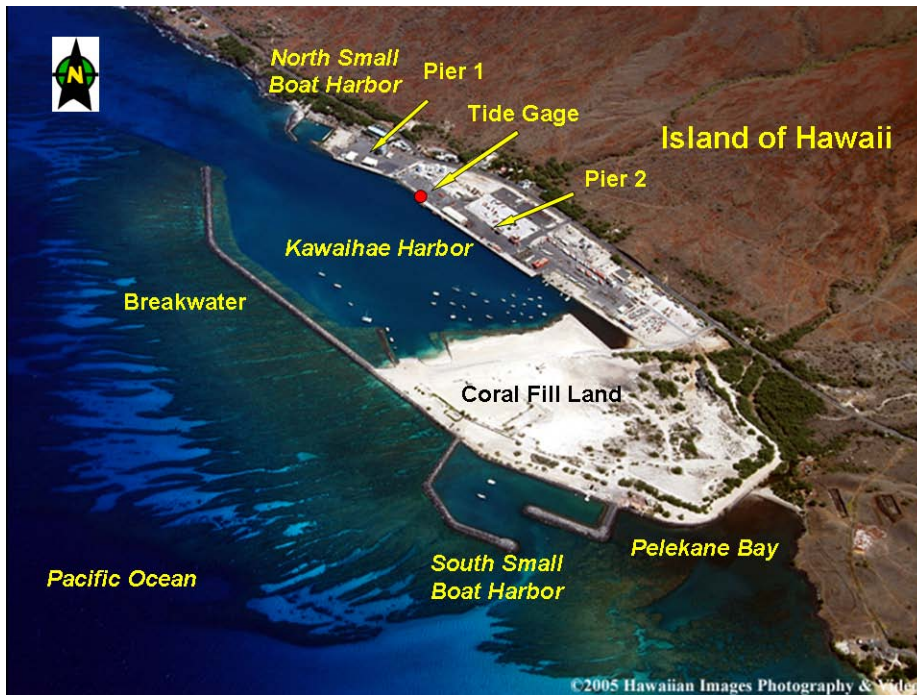
Figure 1. Kawaihae Harbor and Pelekane Bay (Hawaiian Images Photography and Video 2009). The red circle denotes the location of NOAA's Kawaihae tide gage (1617433).
