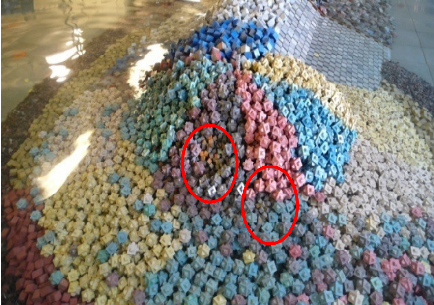
Figure 10. Exposed filter in Cubipod for N_s = 3.2 . 3-D waves, s_{op} = \text{approx. } 0.035 and angle of incidence 0^\circ .
