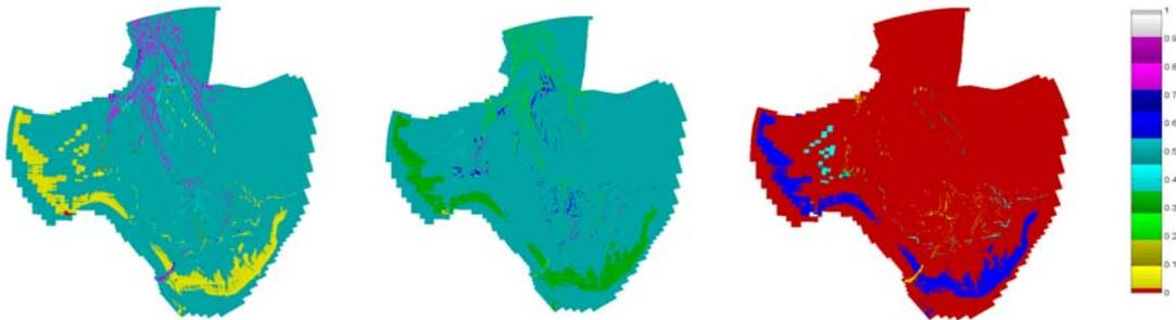
Figure 8. Content of medium sand (left), fine sand (middle) and mud (right) in the second sediment layer at the end of the relocation run.
