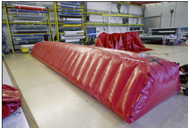
Figure 11. Tube system prototype with inner reinforcements made by the company Karsten Daedler in Trittau, Germany
