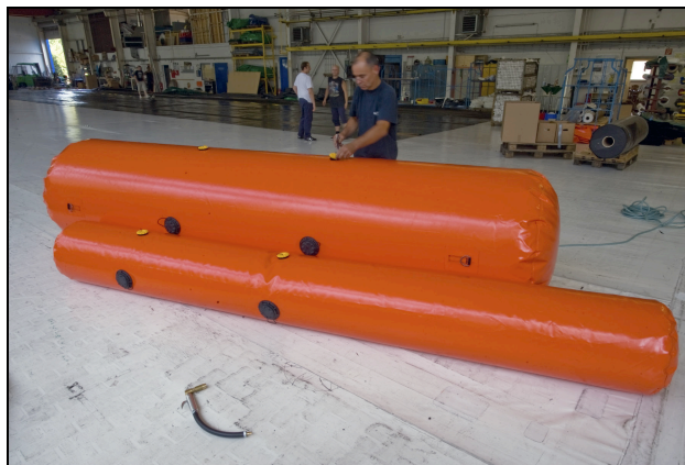
Figure 12. Tube system prototype made of two jointed cylindrical tubes made by the company Optimal in Menden, Germany
