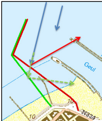
Figure 7 Effect of harbour jetty orientation on wave climate in the harbour
