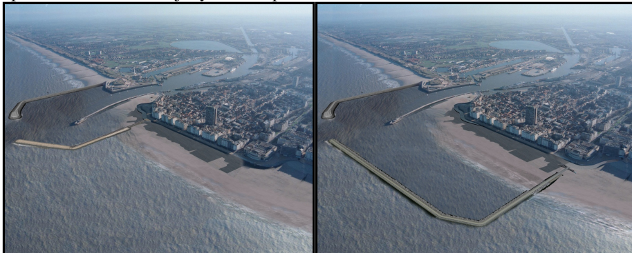
Figure 5: two main options for the harbour jetties: alternative A (short breakwater) and alternative B (long breakwater)
