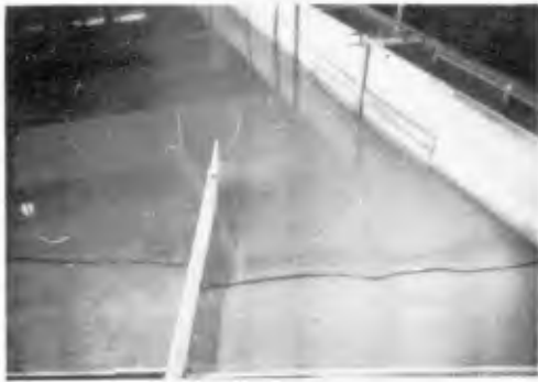
Fig. 24. Laboratory experiment, normal groin, erosion on the lee-side.
