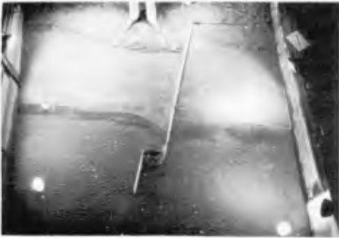
Fig. 30. Laboratory experiment, Z-groin, smooth.
