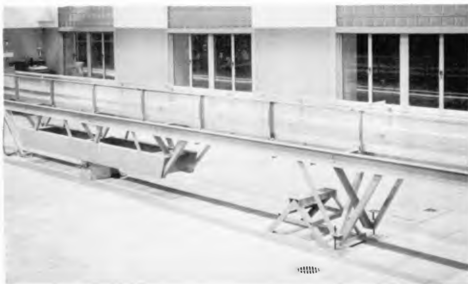
Fig. 2. Wave channel with plunger type wave generator installed.
