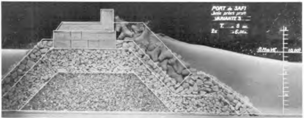
Fig. 4. Study in a wave channel for a revetment made of a double layer of tetrapods.
