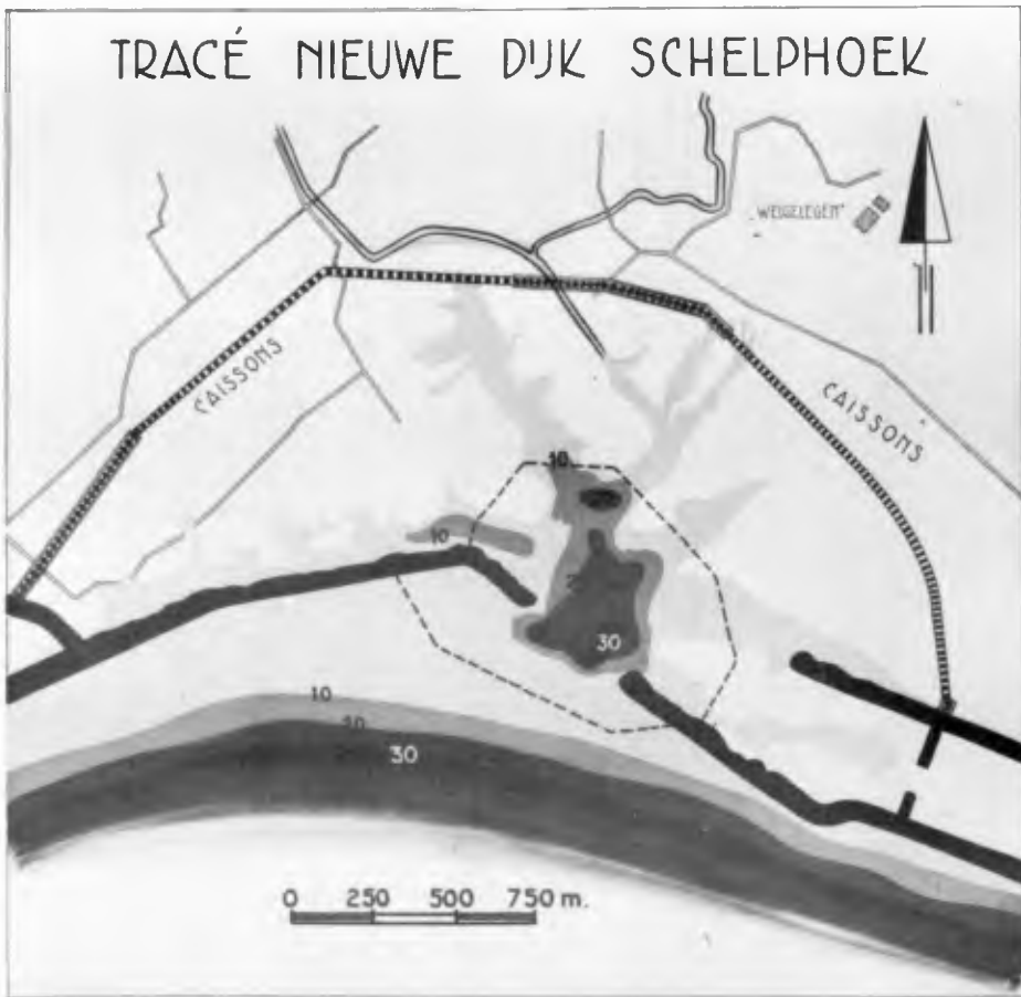
Fig. 12. Alignment of embankment at Schelphoek.
