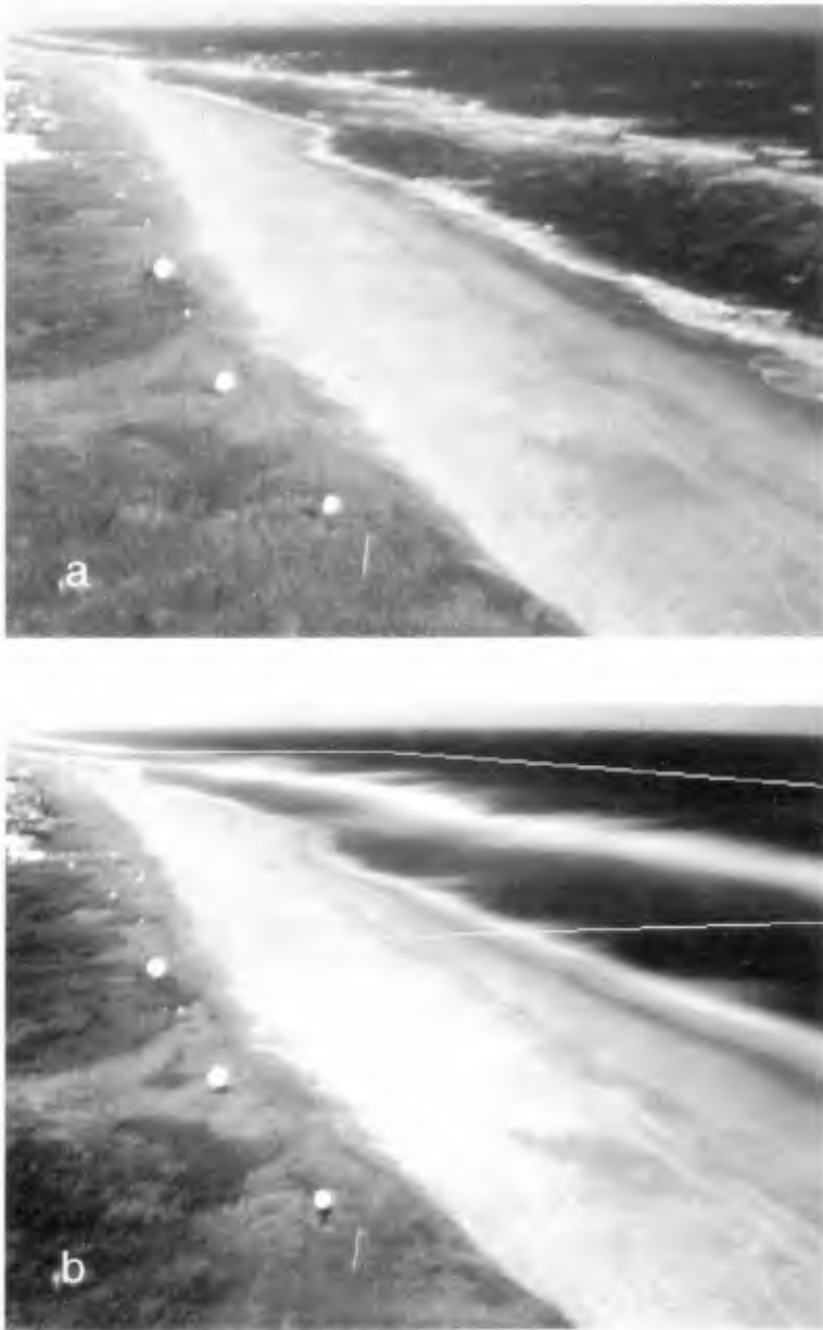
Figure 1. Images from Duck, NC. a). Snapshot from January 10, 1994. b). 10-minute time exposure from January 10, 1994. Transverse features are evident in the trough as well as offshore of the shore-parallel bar. Box shows area rectified in Figure 2.
