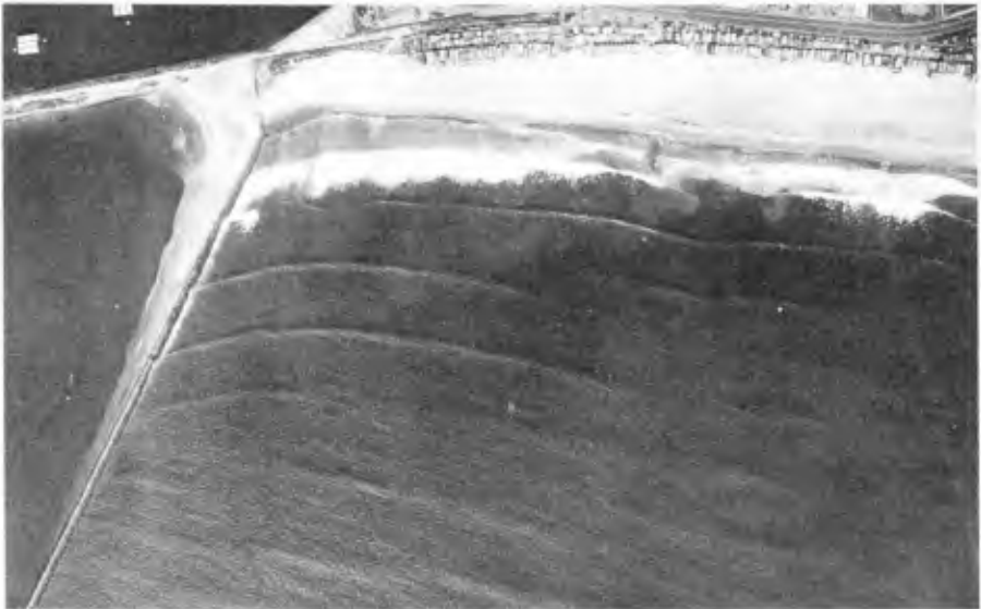
PHOTO 4 Surfside Beach with a West Swell Wave Pattern (April 17, 1981) Sunset Gage: 0904, Hs=110.3 cm; Tp=13s.
