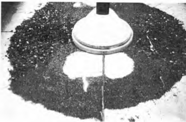
Figure 8 - Scour in Tracer Material for Approach Pier Founded on Seabed
