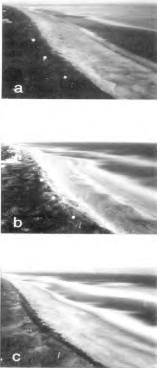
Figure 3. Examples of ratings on a scale of 0-5 that were given to images. a). Time exposure from November 13, 1993. Trough bars were given a rating of 1. b). Time exposure from November 11, 1994. Trough bars were given a rating of 3. c). Time exposure from February 9, 1993. Both trough and offshore bars were given a rating of 5.
