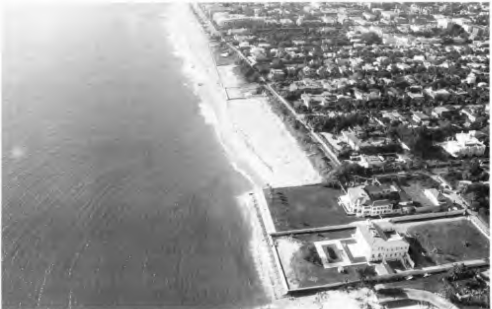
One year after nourishment at Palm Beach, Florida. Photo courtesy of Applied Technology & Management, Inc. and Aerial Photography, Inc.
