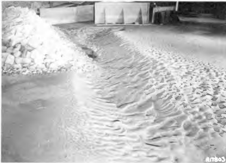
Figure 4: Scour After 10 Hours with 60° Deflection (View from Seaward of Jetty).
