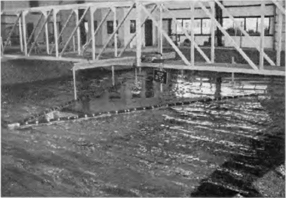
Figure 6. Laboratory Experiment Conducted at OSU Using the Double Delta Version of RIB System with Significant Height = 5 ft, Period = 6 sec..
