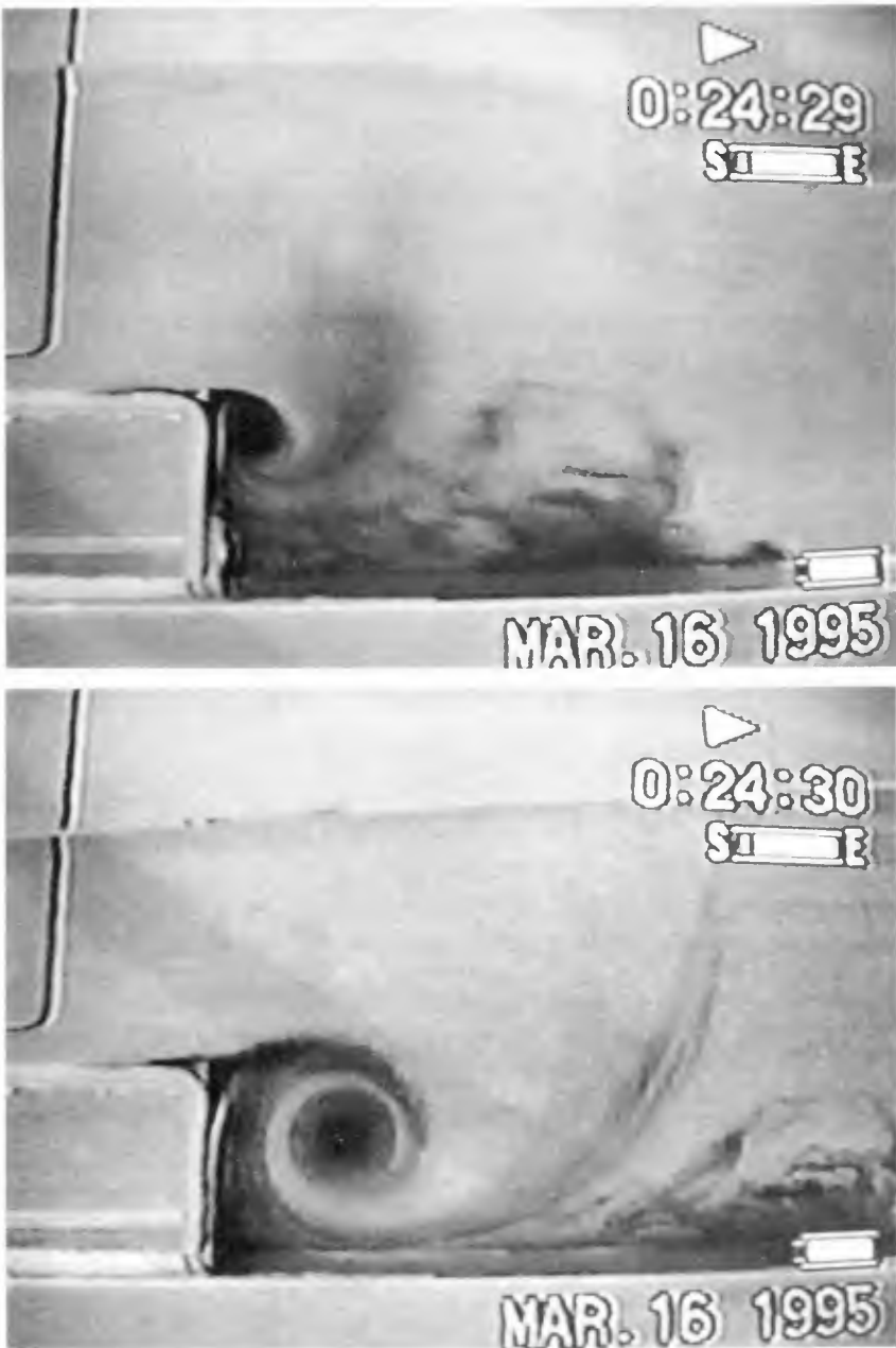
Figure 2: Pictures (A) and (B) of an experimental observation of vortex generation for solitary wave overtopping submerged breakwater. H/d=0.3 , d=9\text{in} , Breakwater C.
