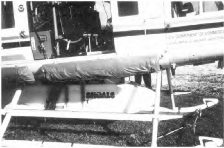
Figure 4: The SHOALS helicopter Lidar bathymetric system. The Pod on the bottom of the helicopter contains the laser, scanner, and optics. The computers and operator's consoles are located inside the helicopter.
