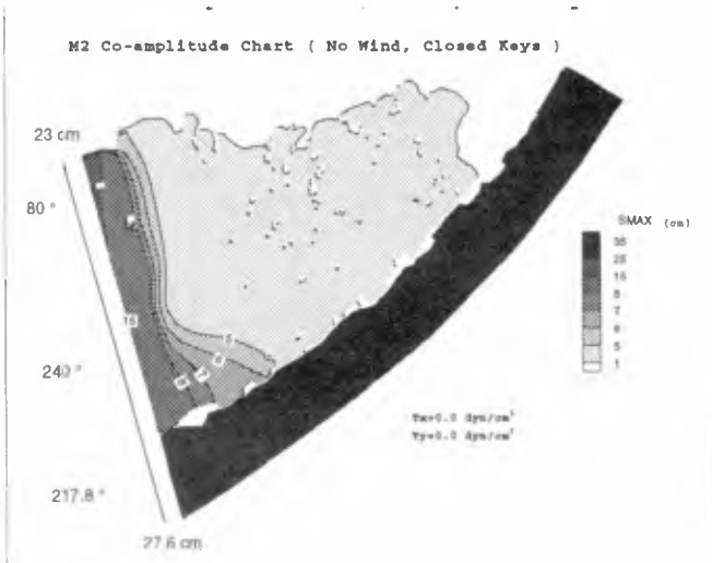
Figure 10. Simulated maximum water level of M_2 tide in Florida Bay with the Florida Keys closed.
