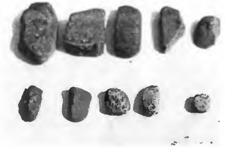
Type 6. Rounded; D_{85} / D_{15} = 1.75 L/D > 2 : 50% L/D > 3 : 15%
