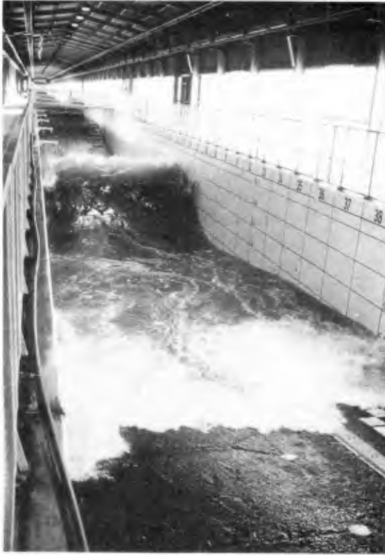
Fig. 2 : Wave action on the revetment during a test in the GWK
